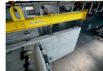
5 Removing cured elements including the butterfly formwork Ta ut de härdade element inklusive fjäril formen
